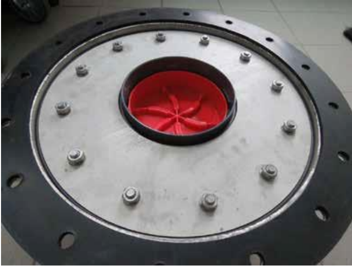
Figure 6: Interior view of the opened test setup with KDS 150
